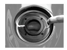
lower installed w/ vent hose
