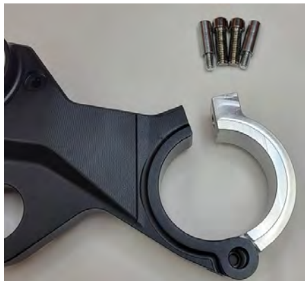
fork leg engagement). (Clamp doesn't have 100% fork leg engagement).
