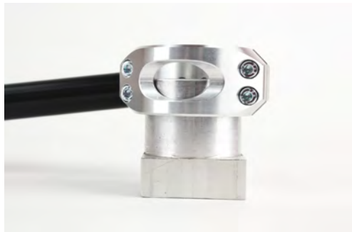
fork leg engagement). (Clamp doesn't have 100% fork leg engagement).
