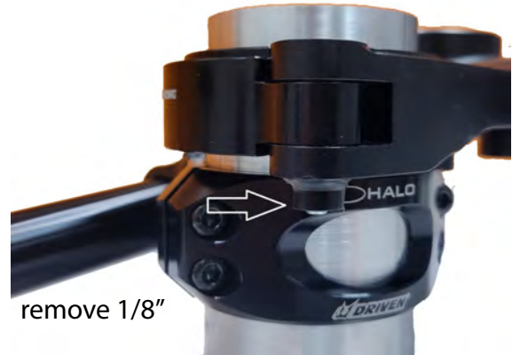
CORRECT (Clamp have 100% fork leg engagement).
