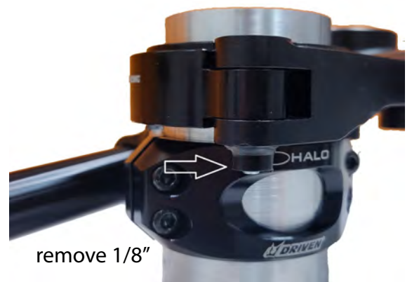
CORRECT (Clamp have 100% fork leg engagement).
