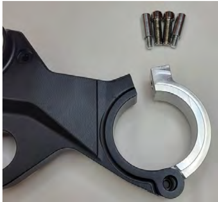
fork leg engagement). (Clamp doesn't have 100% fork leg engagement).
