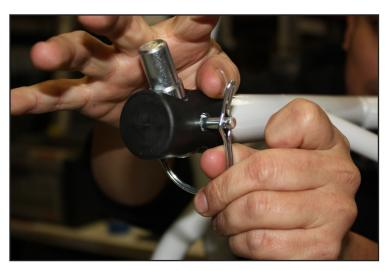
\*Head Lift Stand must be used in conjunction with the Rear Stand. With the stand assembled and the bike sitting on a Rear Stand, push the pin into the stem. Lower the stand and lift the bike.
