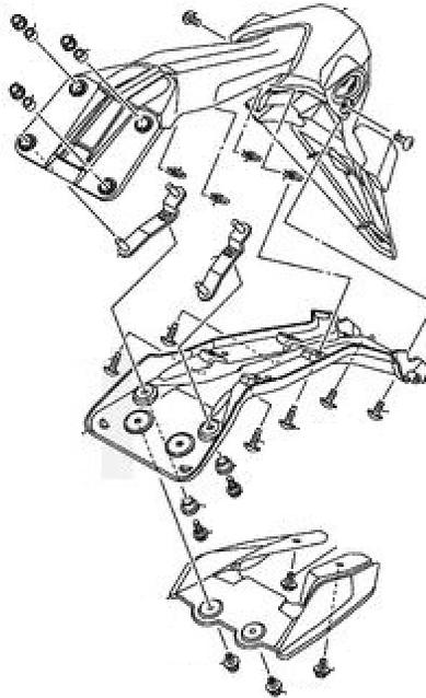
**THE USE OF BLUE LOCTITE IS REQUIRED ON ALL MOUNTING HARDWARE!**
