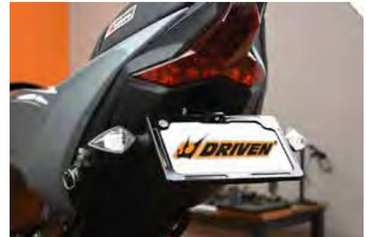
**THE USE OF BLUE LOCTITE IS REQUIRED ON ALL MOUNTING HARDWARE!**
